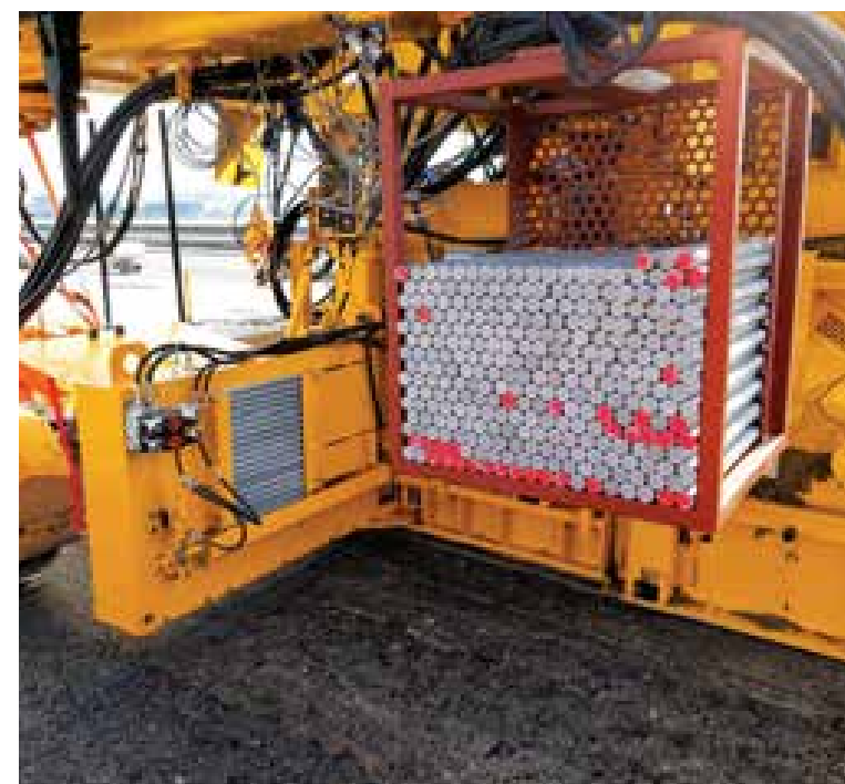
The hydraulic powered magazine-style side bar inserter allows personnel to load multiple bars into a magazine clip. The bar inserter then releases a single bar and places it at the specified distance.
