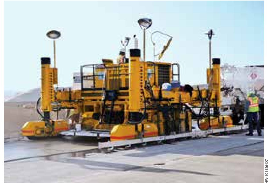
A GP-2400 paves a 0.75 inch (19 mm) thick polymer overlay on a new bridge deck.
