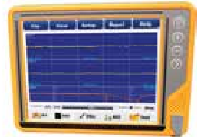
The Navigator's GSI trace screen showing the simulated California profilograph graph.
