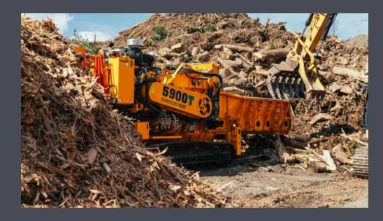
Designed as the first generation of the 5900, this machine combines the best of both worlds, blending features from the traditional 6800 and the 5800. With its 60" wide infeed rotor, the 5900T significantly enhances material flow, effortlessly handling wider material and reducing the need for pre-processing. Its 8'6" legal transport width and redesigned dolly system enhance mobility and transport efficiency, while
