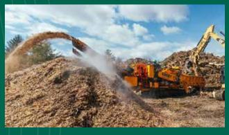
ENHANCED DISCHARGE SYSTEM WITH WEAR PLATES AND OPTIONAL METAL-EJECTING PULLEY—BUILT FOR ULTIMATE DURABILITY AND PERFORMANCE IN TOUGH JOBS.
