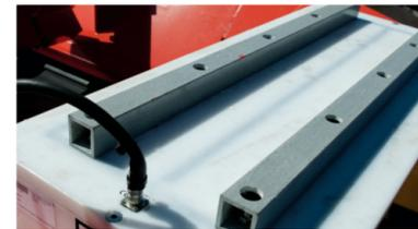
Bridge coil metal detector for controlled detection
