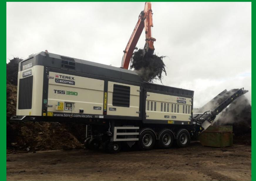
The TSS 390's 3m long shredding shaft was expertly designed in-house and is made from heavy-duty steel, with easily replaceable, bolt-on shredding teeth. Being hydrostatically driven, it offers the benefit of full speed, full torque reverse as well as protection against contaminants. Customisable shredding programs enable the operator to configure the machine to their specific requirements and offers improved shaft cleaning in difficult applications, reducing wrappage and optimising throughput.
