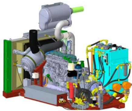
A powerful Scania engine with a low operating speed combined with an efficient hydrostatic drive creates a very responsive shredding action with protection against unshreddable contaminants and also offers full torque, full reverse
