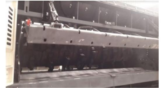
Hydraulically operated access doors on both sides of the chamber for teeth replacement and servicing
