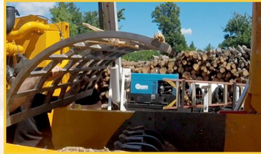
60" wide cleated discharge belt provides unrestricted discharge of ground product.
