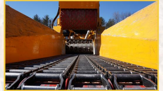
Infeed walls wing outwards to increase loading clearance and funnel material.
