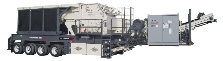
Note: Unit shown with optional electrical panel and hydraulic leveling jacks.
