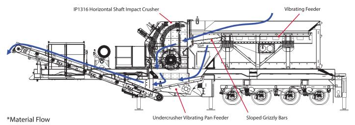
\*Unit shown with optional electrical panel and hydraulic run-on jacks.
