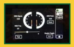
A problem for any industrial grinder has to do with tramp metal entering the hog box and causing significant damage, which leads to downtime. The Metal Detection System™ (MDS) engages within milliseconds whenever the grinder's rotor makes contact with tramp metal.
